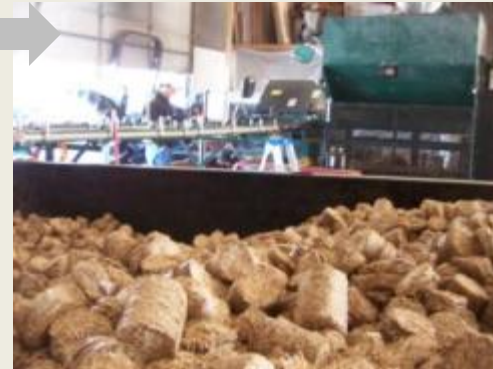
RER Compacting Switchgrass into Briquettes
